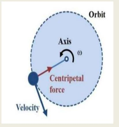
• Centrifugation is a technique of separating substances which involves the application of centrifugal force.The particles are separated from a solution according to their size, shape, density, the viscosity of the medium and rotor speed.
